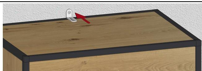
Mounting the tilt protection for highboards
